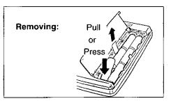
Replace the batteries when blinking mark " \( \sum \) " appears on the player's display.
