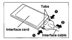
Pull the Interface cable straight while pressing the side tabs of it.
